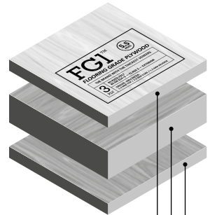
1.3mm FACE 3.3mm CORE 1.3mm REVERSE
